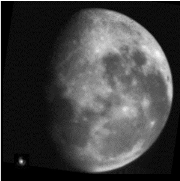
Figure 1. The moon imaged at Steward Observatory with the first telescope to use a primary mirror of Stretched Membrane with Electrostatic Curvature (SMEC). The silicon nitride membrane was 0.7 \mu\text{m} thick and curved to a 3 m focal length by a field of 2 MV/m. A 6 mm stop was used to obtain diffraction limited image quality, as shown by the Airy pattern of the star image inserted bottom left.
