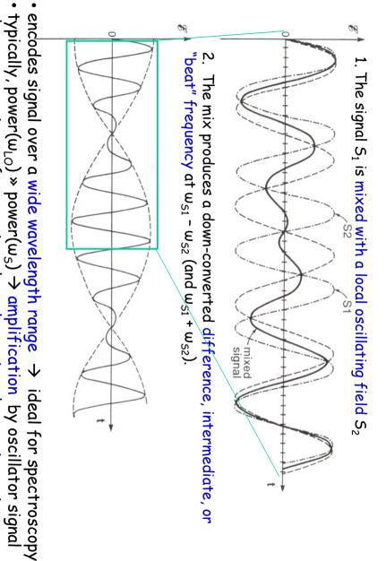
down-conversion to frequencies where low-noise electronics exist
