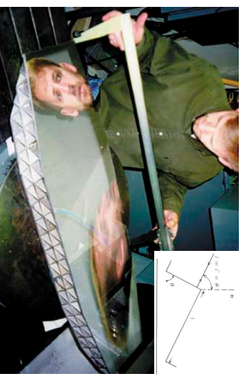
The ruled echelle grating of the SOFIA Facility Spectrometer ARIES. Two images of the engineer are seen reflected from the facets of the grooves that are at angles of 90 degrees from each other.
