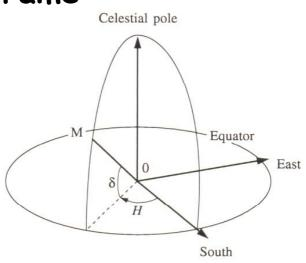
Fig. 8.3. The hour system of coordinates
