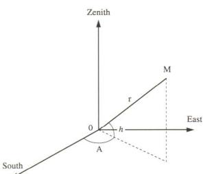
Fig. 8.2. Definition of the horizontal reference system
