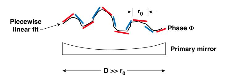
The number of subapertures is  $(D/r_0)^2$  at the observing wavelength  $\rightarrow$  can easily require hundreds to thousands of actuators for very large telescopes.
