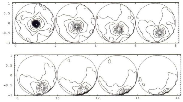
Motion of a frozen patch of atmosphere across the 3.6m telescope aperture. Pictures by E. Gendron (1994)
