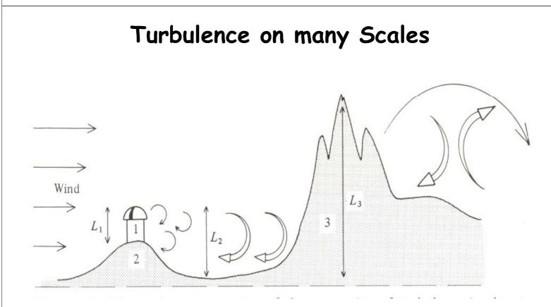
The scales L1, L2, L3 are characteristic of the outer (external) scales of turbulence caused by the wind around the obstacles 1, 2, 3.
