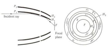
Fig. 4.33. Side and front views of a Wolter X-ray telescope. P and H denote parabolic and hyperbolic surfaces of revolution, whose common axis points to the source
