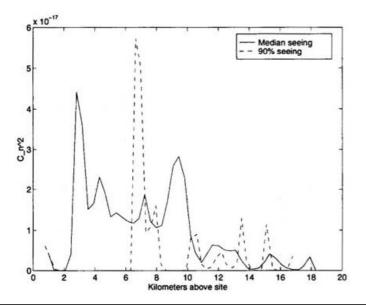
Median seeing conditions on Mauna Kea are taken to be  $r_o \sim 0.23$  meters at 0.55 microns. The 10% best seeing conditions are taken to be  $r_o \sim 0.40$ meters. Figure taken from a paper by Ellerbroek and Tyler (1997).
