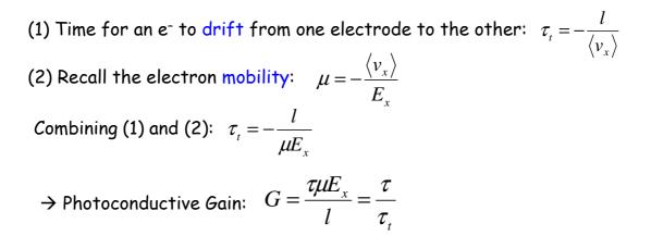
au is the mean carrier lifetime before recombination. Hence: The photoconductive gain is the ratio of carrier lifetime to carrier transit time.
