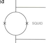
If the SQUID is biased close to  $2I_0$  very small changes in I can be detected at the SQUID output (acts as a low input impedance amplifier).
