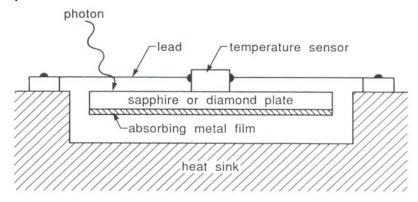
The heat capacity of the blackened sapphire plate is only 2% of that of Ge.
