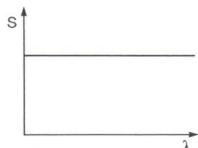
Note: The bolometer responsivity is independent of the wavelength of operation (as long as the QE  $\eta$  is independent of  $\lambda$ )
