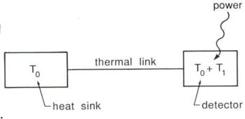
Now we add an additional, variable component  $P_V(t)$  =(astronomical signal)  $\rightarrow$  the temperature will change, according to
